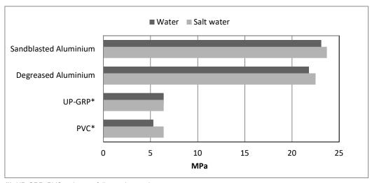
(\*): UP-GRP, PVC, substrate failures observed.
