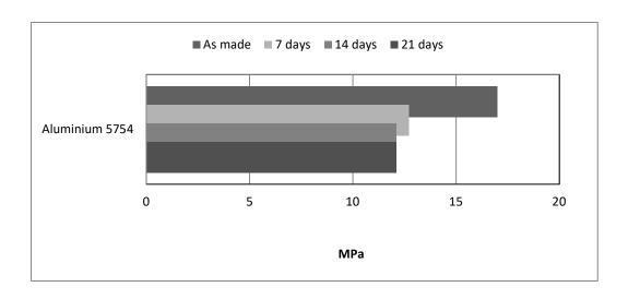
Lap shear strength after coating post-cure cycle at 200°C (typical average values)
