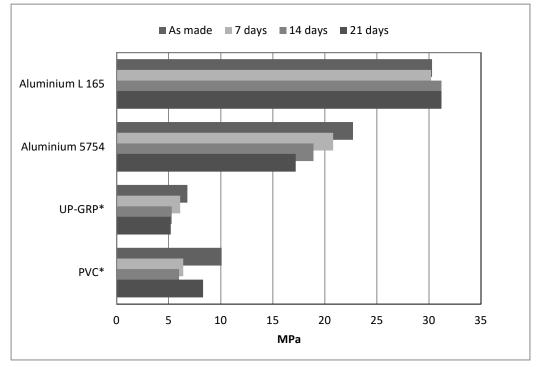
(\*): UP-GRP, PVC, substrate failure
