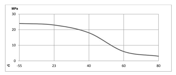
Roller peel test (ISO 4578) (typical average values) On etched aluminium
